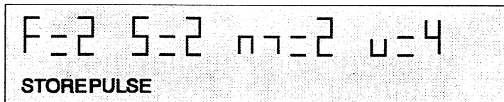
Figure D35. Display status in the ringer programming mode.
