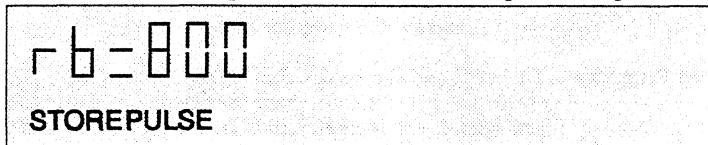
Figure D29. Display status at set impedance Rb, showing the Rb value of 800 ohm.
